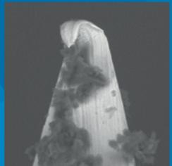
Electron micrograph images of 27G needles (1000x magnification) after injection into mice demonstrating the potential for dulling of the needle and contamination when reused.
